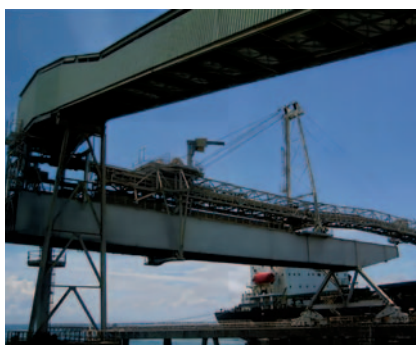
Belt tracking keeps loads centred and minimizes dust from spillage and disruption.
