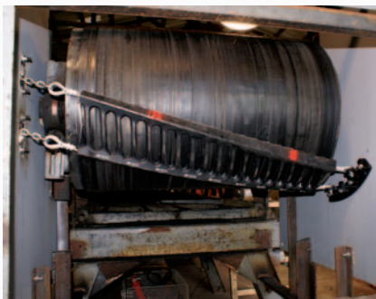
The low-profile Cleanscape primary cleaner takes up less space than standard cleaners. © Martin Engineering 2024
