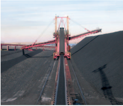
Port terminals of coal or petcoke with exposed stacker conveyors can be especially vulnerable to dust emissions. © Martin Engineering 2024
