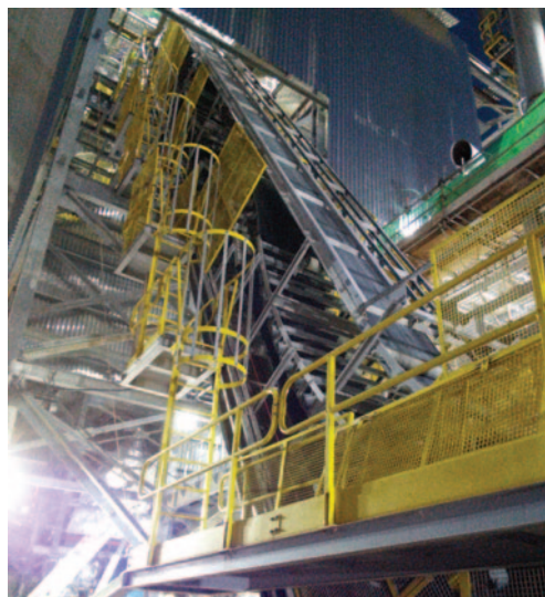
The DSI Sandwich Belt high angle conveyor offers a small footprint, elevating 720tph of limestone, iron ore, sand and clay at a 60° angle.
