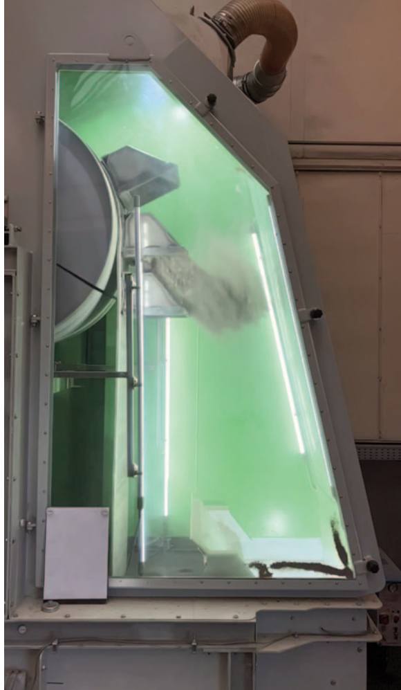
Figure 2: Digital DEM mapping (left) and field test of the bucket elevator in Beckum, Germany (right).
