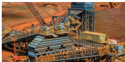
NextGen modular crushing plants that produce significantly lower dust and noise emissions than traditional crushers.
