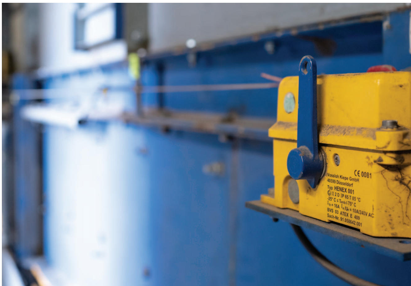
One of several pull-rope emergency stop switches from Kiepe Electric at E.ON. Regardless of how often the pull rope has had to be pulled during operation of the conveyor belt, the switches are still functional even after more than a decade.
