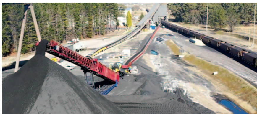
Train unloading and stockpile management of coal with MCS specialized conveying equipment.
