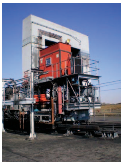
DemcoTECH's recommendation for upgrading and enhancing of the coal off-loading and delivery system for a South African power utility included the tandem wagon tippler.
