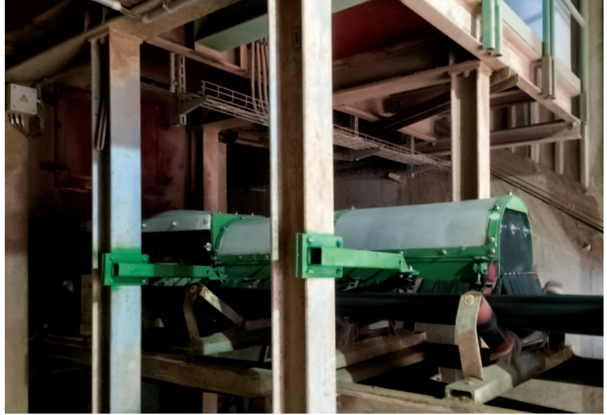
The DustScape dust filter system, which is used in conjunction with the contact-free AirScape conveyor belt skirting system, has been specially developed for the control of dust formation and material spill at critical sections along the conveyor route and transfer points.
