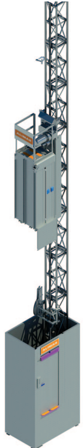
Alimak Group's SE 240L elevator, designed for installation on silos, storage vessels, cranes and other industrial applications, eliminates the need for a machine room or a supporting elevator shaft, reducing building requirements and ongoing structural maintenance.
