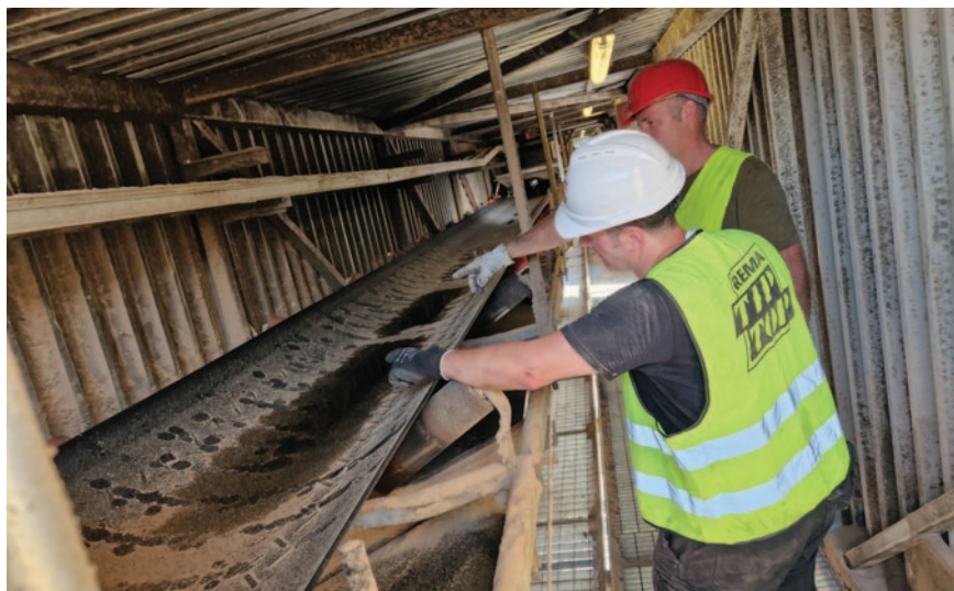
The REMA TIP TOP experts select a special conveyor belt profile for optimum material transport of the moist woodchippings.
