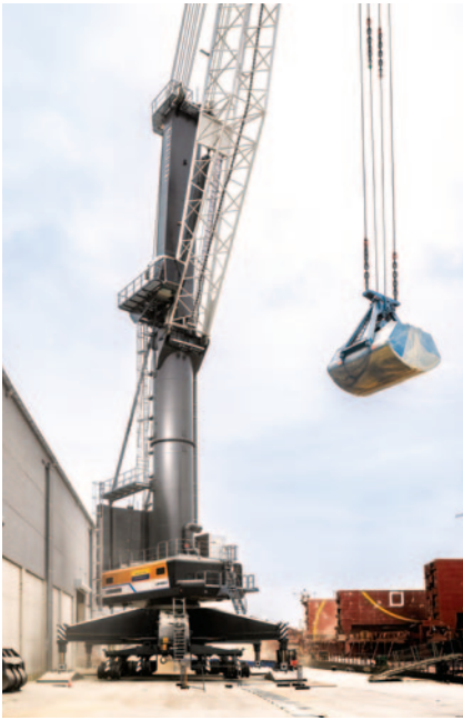
The Liebherr LHM 800 mobile harbour crane, at Marcor Stevedoring's Hartel Terminal in Rotterdam, has a lifting capacity of up to 144 tonnes.
