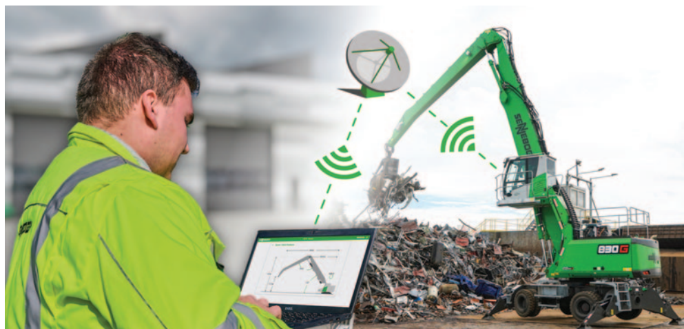
The new SENNEBOGEN control system SENcon creates the basis for the long-term technological further development of the machines through its intelligent networking and communication capability.
