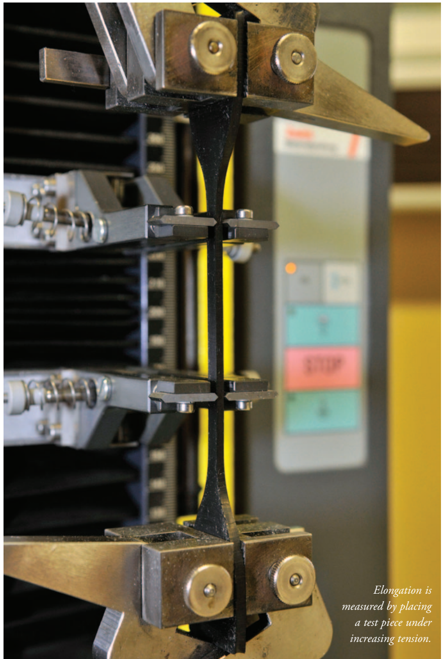
Low elongation can cause stress that leads to delamination.
