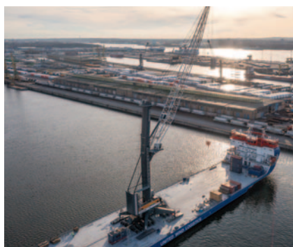
A milestone for Marcor and Liebherr: This LHM 800 is the first crane of its kind to operate with an all-electric drive system. With its 64-metre reach and peak dry bulk operating capacity exceeding 2,000 tonnes per hour, it perfectly aligns with Marcor's bulk, bagged and containerized stevedoring operations.
