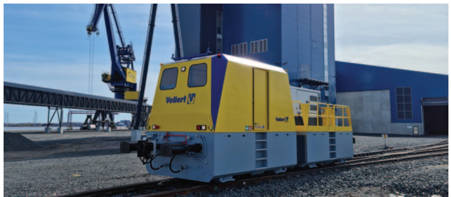
Olmar Management B.V uses robust technology from Germany for rail loading of bulk goods in Pori, Finland: the radio-controlled shunting robot Tandem DER 150 from Vollert has a flexible coupling for Eastern and Central European wagon systems as well as a hydraulic unit for opening the wagon roofs. Source: Vollert
