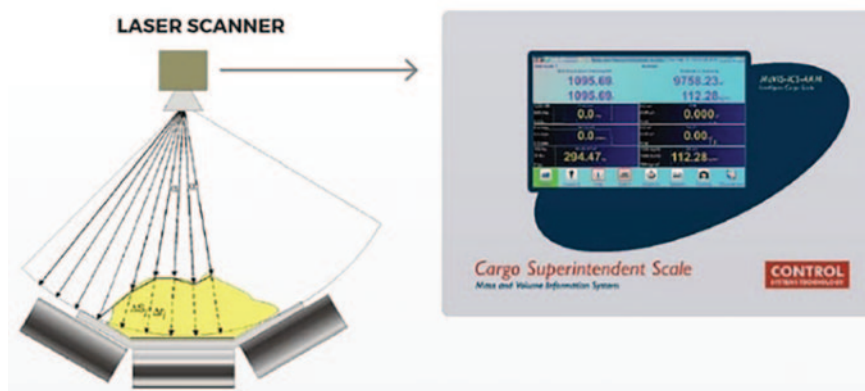
CST's Volumetric laser scanner system allows real time monitoring of surcharge angles, material volume and material edge margins.
